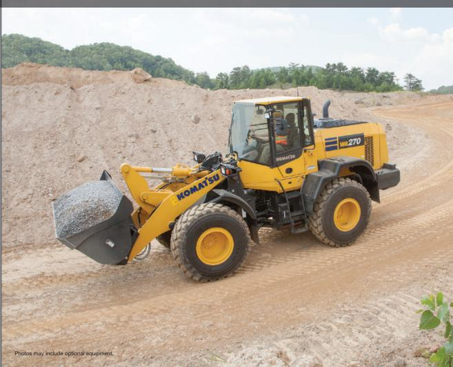
NET HORSEPOWER 149 HP @ 2000 rpm 111 kW @ 2000 rpm
